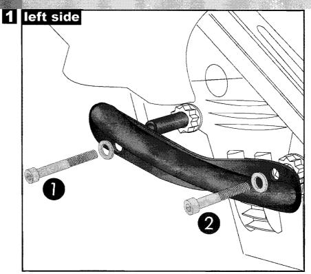
Fastening of the engine guard right: at the two upper points of the engine suspension. Original screws are obsolete.
