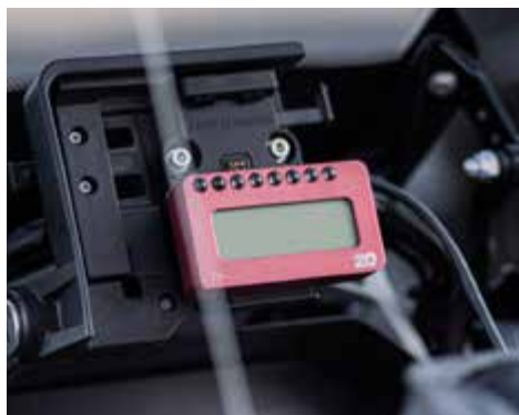
Real-time data display: displays the can-bus and the data of the sensors and the GPS system
