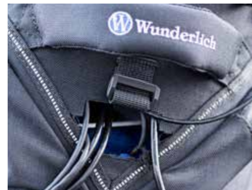
ELEPHANT tank bag as a black box: data recording, GPS system and the interface to the can-bus system are housed here
