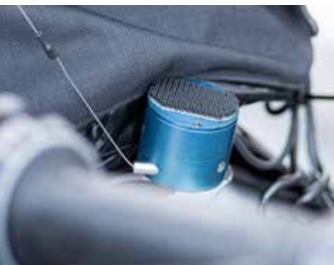
Displacement sensor for recording the deflection of the windshield under a wide range of ambient and load conditions
