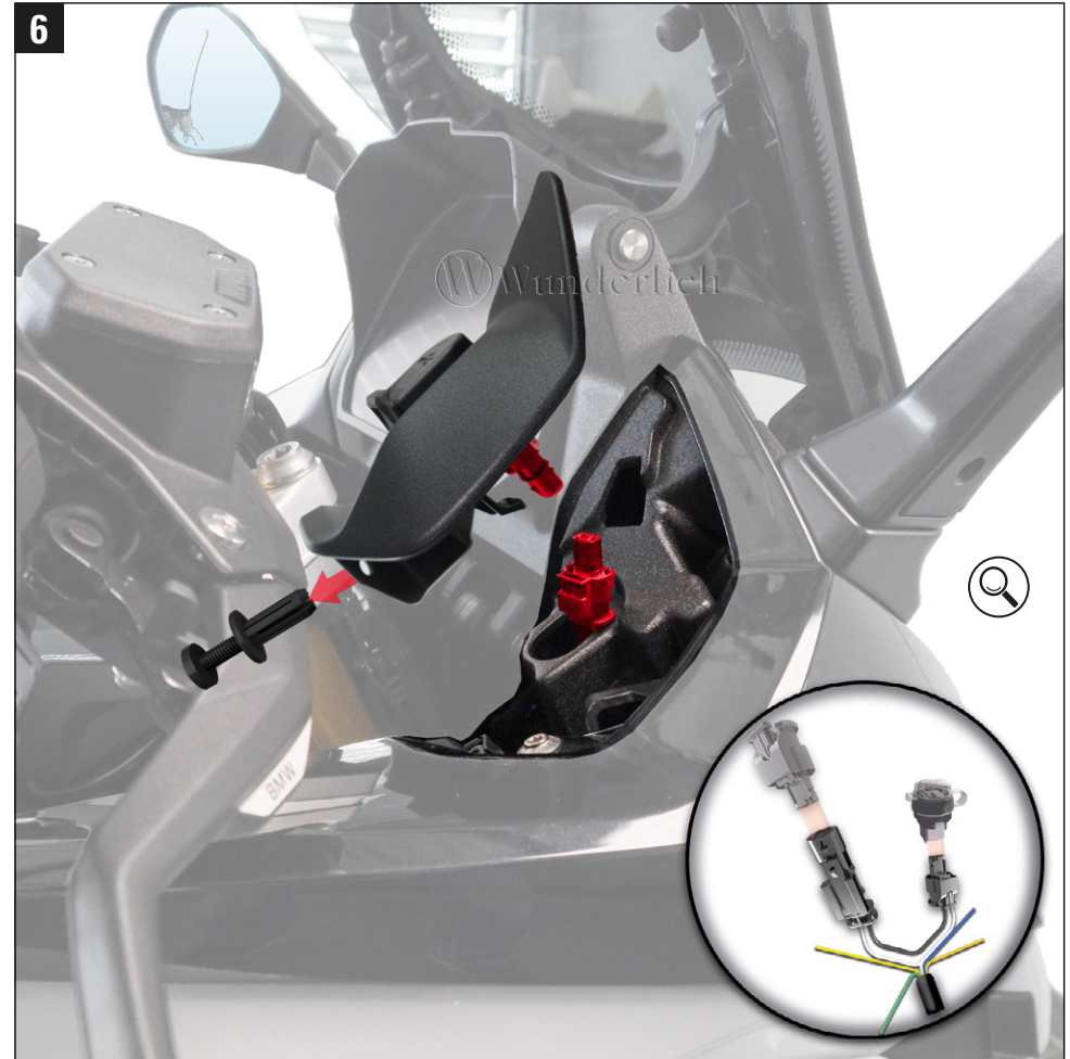
After connecting the MICROFLOOTER, the tank cover is reassembled in reverse order.
