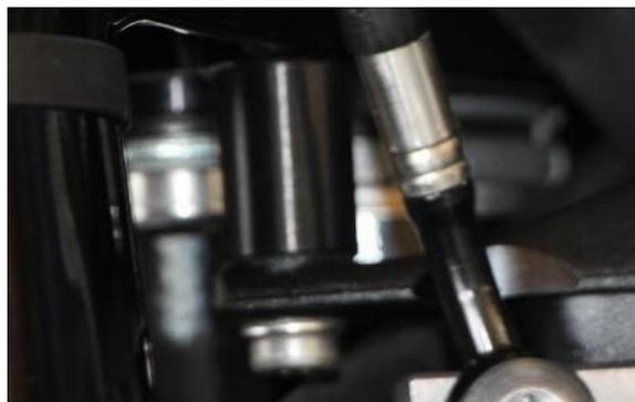
Loosen the speedometer holder and attach using the spacer bushings, washers and screws provided.
