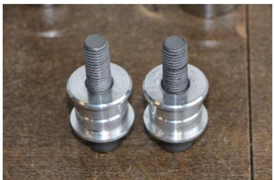
Remove the original screws and bushings.
