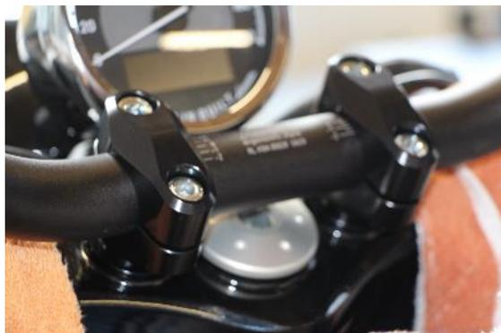
**Caution: The narrow side of the risers must be aligned towards the driver.**
