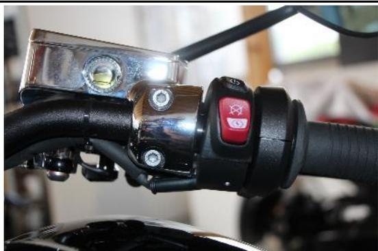
Reconnect the plug connectors of the handlebar switches.
