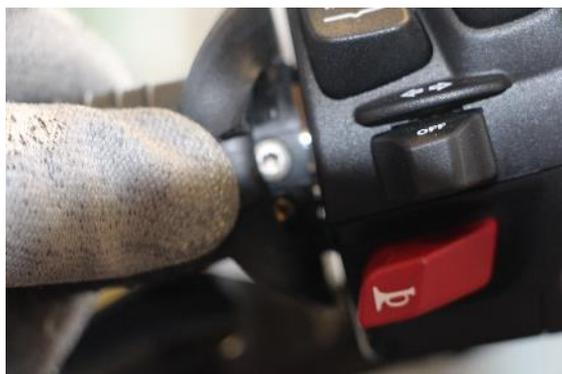
Dismantle the housing of the switch units on both sides, loosen the fixing screws and unplug the plugs of the units.
