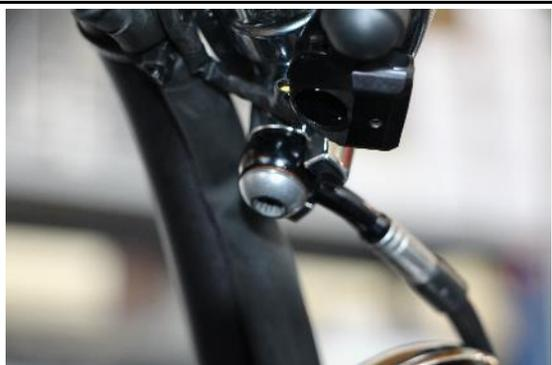
Attach the brake and clutch lines provided to the pumps and manifolds.
