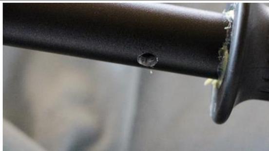
The final assembly of the operating elements requires the drilling of holes for the centring pins. To do this, align the operating elements and mark the positions for the centring pins (push onto the pins using grease). Now, centre-punch the marked position and drill a hole (diameter and depth are based on the centring pin).
