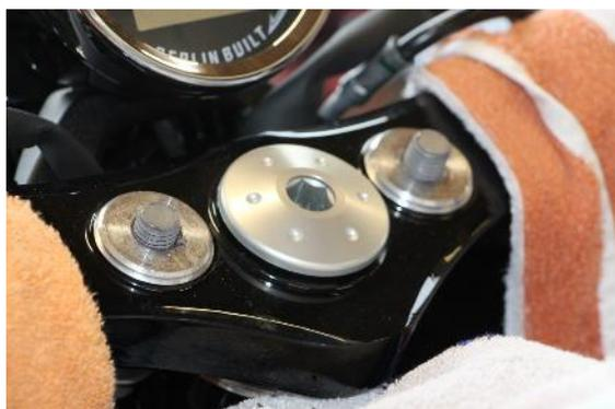
Remove the two screws under the top yoke, pull the cable harness out of the handlebar and remove the handlebar with the risers.
