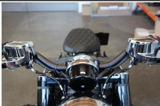
After the final assembly, check the freedom of movement of all brakelines and cables and fasten them only to such an extent that they are not bent, do not chafe and are tension-free in maximum steering angle and over the entire spring travel.
