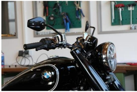
Fasten all screws with thread-locking fluid (medium strength) and the preset tightening torque.
