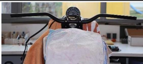
Insert the handlebar back into the risers, adjust as desired and fasten.
