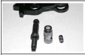
Unscrew the push rod from the guide pin and remove both parts from the original adapter.
