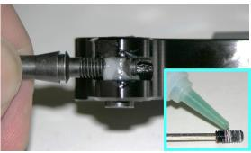
Moisten the plastic bushing of the guide pin with grease and insert into the new adapter as per original (thread for the safety screw facing downwards).
