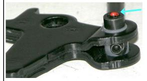
Lightly heat the safety screw using a heat gun (thread-locking fluid) and remove.
