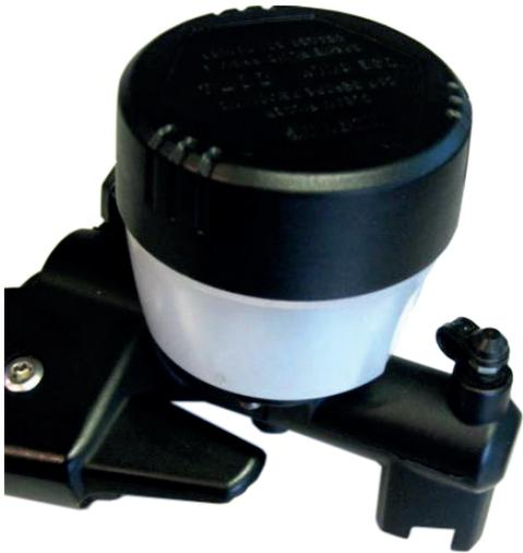
Wunderlich-Brakeboxes are only suitable for BMW- Motorcycles with Integral-ABS Generation 2, which are equipped with a direct mounted, round plastic brake fluid reservoir on the master cylinder. The master cylinder has also to be provided with a bleeder. Please also compare adjoining illustration.
