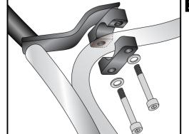
Fastening of the tank guard left and right bottom:
