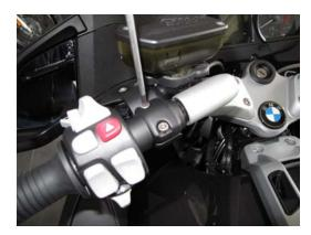
1. Remove top clamp of lever perch.
