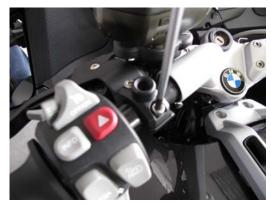
2. Install Mirror adapter and tightem bolts
