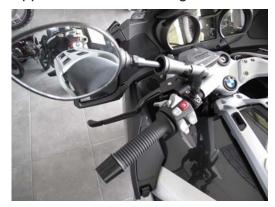
4. Pull back the rubber boot of the Flash mirror to access the length adjustment nut.
