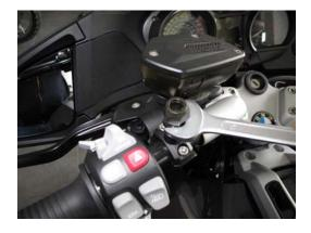
3. Screw in the base adapter(s) supplied with the Flash mirrors and tighten with a 17mm wrench. If different mirrors are being used, attach them to the adapters instead.
