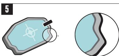
Align the screen protector onto the dashboard. The water/soap solution will allow you to move the screen protector until it is lined up correctly. Note that most of our protectors allow a small gap around the edge to prevent it from lifting, so please align the screen protector in the centre
