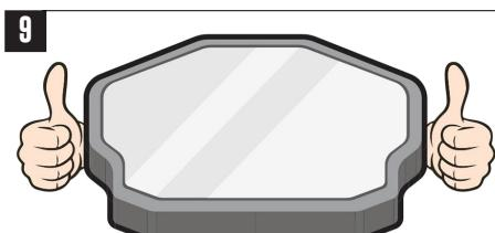
Don't worry if you see small bubbles/water under the protector after fitting, use your squeegee to remove these and any remaining bubbles should disappear within 1-2 days
