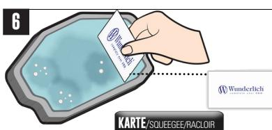
Gently squeeze water and air pockets out with the squeegee. Try to remove as much water and air bubbles as possible but ensure you are gentle to prevent the screen protector from moving
