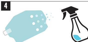
With the liner removed spray a liberal amount of water on the side you have removed the protective layer from. Try not to touch the adhesive to prevent finger prints
