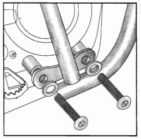
Fastening of the engine guard bottom:
