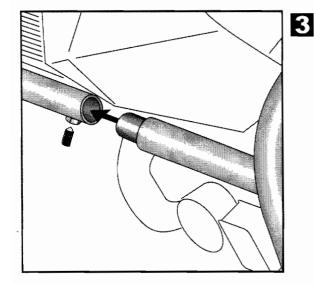
When assembling the right engine guard it must first be connected to the left one.
