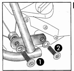
Pastening of the engine guard bottom:
