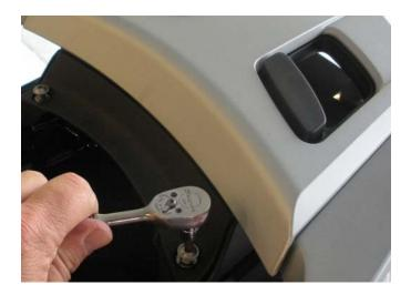
Remove the luggage rack. Two screws on each side, two screws under the passenger seat
