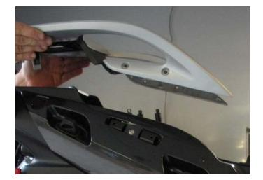
.....two screws at the rear, accessible after removing the tail light. Remove the luggage rack.
