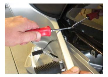
Remove the three screws from the fairing panel, carefully bend the panel back to expose lower side panel attachment screw and remove that screw.
