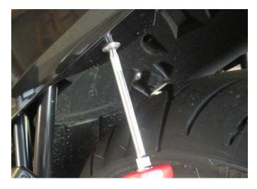
Remove the screw where the luggage rack was attached. Remove the screw on the under side of the side panel.
