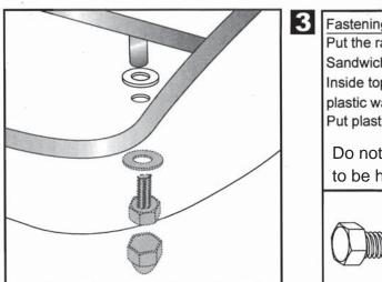
Fastening of the railing front:Put the railing on the top case cover over the borings.Sandwich the rubber washers Ø 7 x Ø15 x 3 mm.Inside top case cover use the hexagon screw M6 x 20 withplastic washers Ø18xØ7x1,5.Put plastic caps on the screws head.Do not overtighten fasteners! The screws only needto be hand tightened. Thread locking fluid recommended.Image: AxImage: AxImage:
