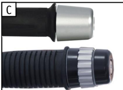
2. Insert the bar weight (CruiseControl) assembly into the handle bar end (Image B). Hold the bar weight (CruiseControl) and tighten the bolt.
