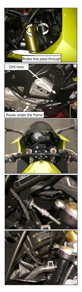
Attach the short brake line to the Sportego fork bridge with the supplied banjo bolt, crush rings and route it as shown in the image. Attach to the front brake master cylinder using the original banjo bolt and new crush washers. Attach the original brake fluid reservoir using the supplied bracket, attached to the upper perch of the brake cylinder. The brakes must be bled in accordance with BMW procedures and specifications.
