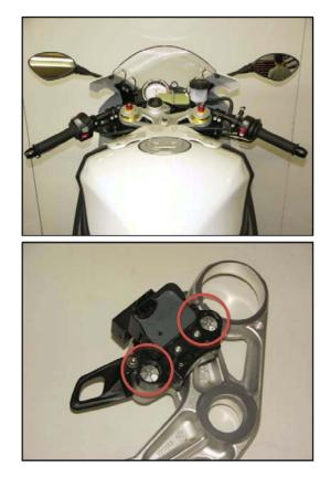
Attach the ignition switch assembly, spacers and ignition switch ring to the new fork bridge with the supplied screws and torque to 18-21 NM (13-16 ft/lbs)
