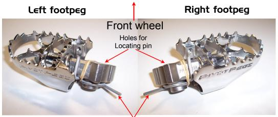
These lean against the motorcycle frame and are compressed when pegs are moved into position and locating pins are inserted.
